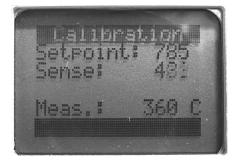
If you want to use your own soldering iron instead of the one your PortaStation came with or just want to make sure your iron is well calibrated you can always calibrate it by using the wizard located in
